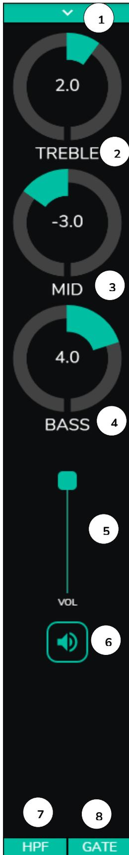
1. Drop-down menu showing the options for POLARITY, STEREO, FREQUENCY SHIFTER and LABEL edition.
