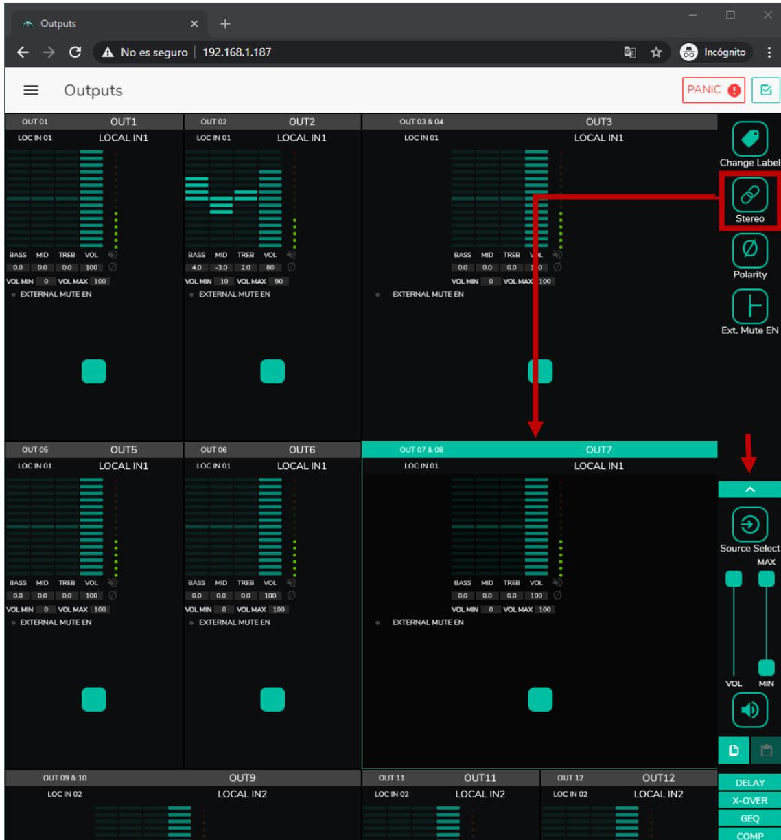
Figure 35: outputs configured as a stereo pair
