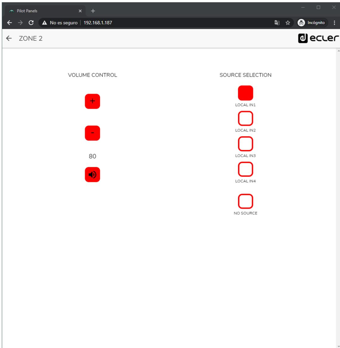
Figure 58: *pilot panel* with volume control and source selector
