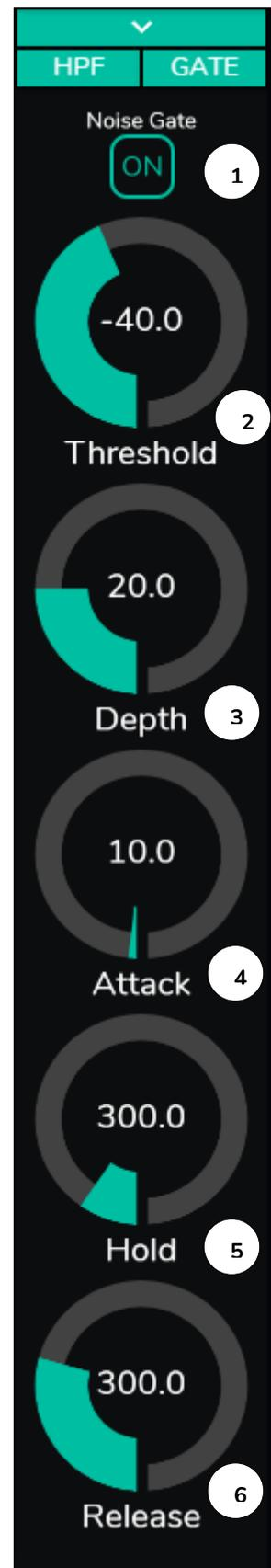
Figure 31: noise gate configuration of an input
