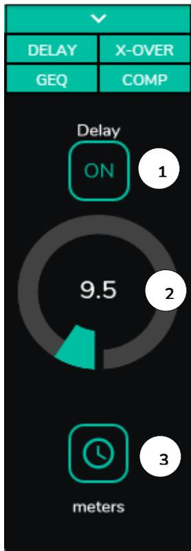
It allows the adjustment of a delay in milliseconds, meters or feet, to be applied between its input and output. It is independent for each output. Useful to adjust sound reinforcement systems that use reinforcement speakers far from the main system and avoid delaying signals to the audience. Available for outputs 1 to 8 in all HUB devices.
