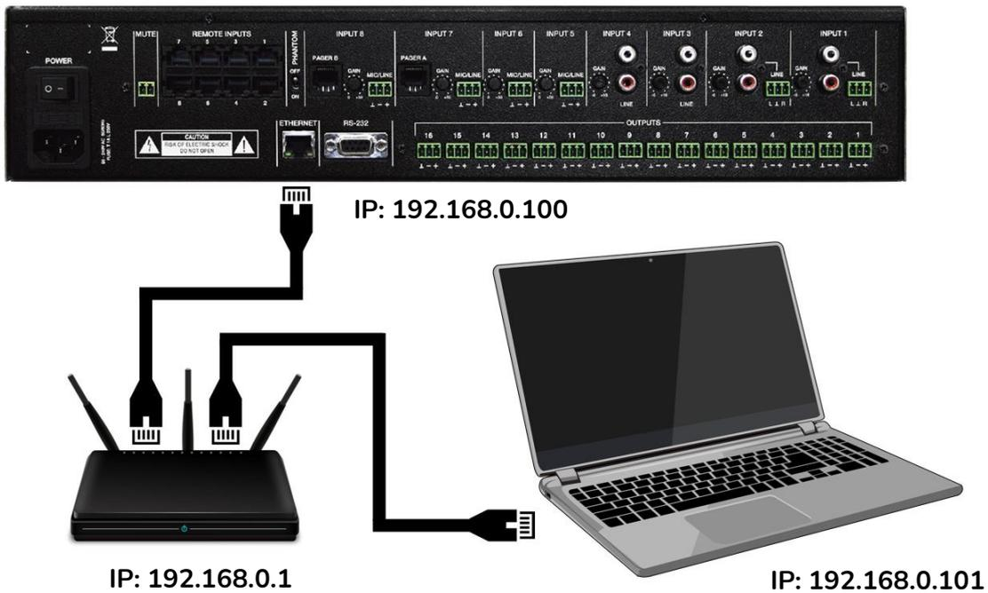
Figure 3: LAN local network connection
