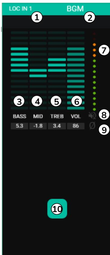
1. Local input indicator, connectors on the rear panel (LOC) or remote (REM), remote control panels with audio input, plus the corresponding numbering.
