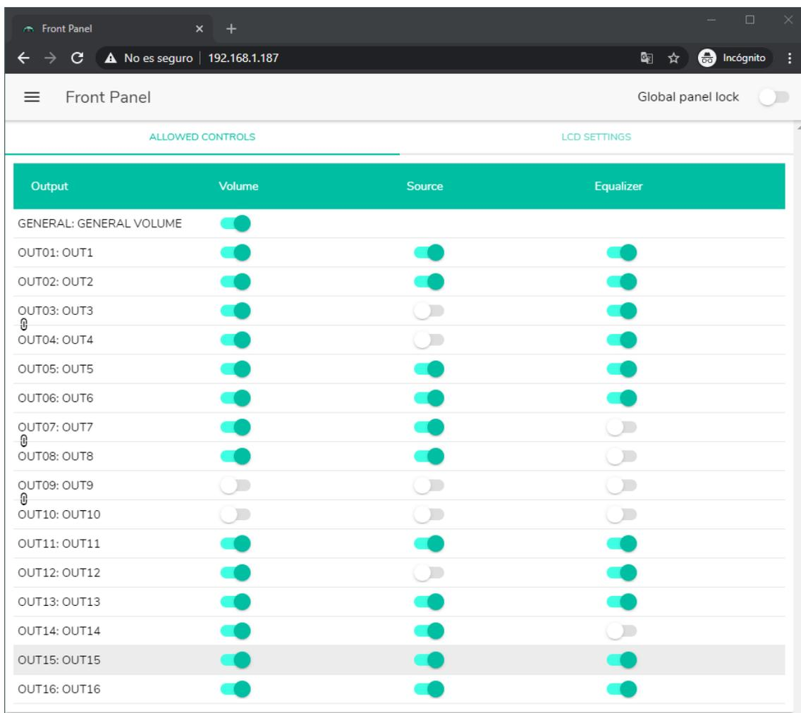
Figure 17: allowed controls on the frontal panel
