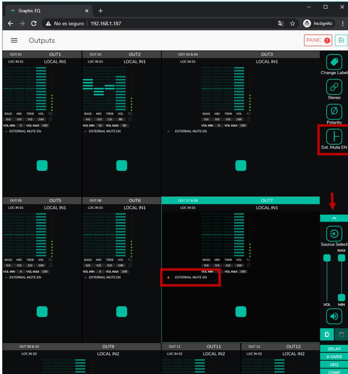
Figure 36: activation of external mute by contact closure on one output
