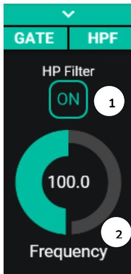
Useful for attenuating the proximity effect of a microphone (boost at low frequencies) or eliminating/attenuating background noise, handling noise, etc:
