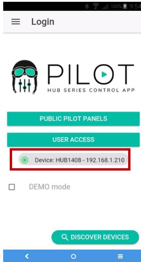
Figure 67: HUB device connection status
