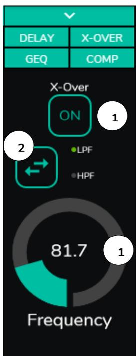
Allows you to insert a crossover filter (low pass or high pass) on the selected output. It is independent for each output. Useful if you connect a sub-bass to this output, for example. Available for outputs 1 to 8 in all HUB devices.
