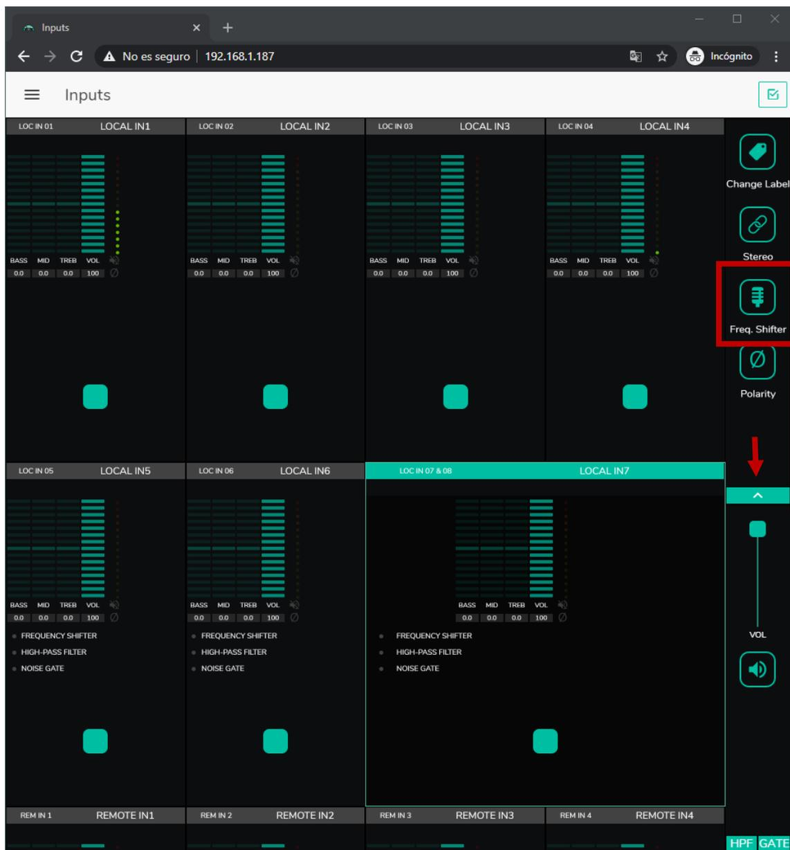
Figure 28: enabling the feedback canceller (FREQUENCY SHIFTER)
