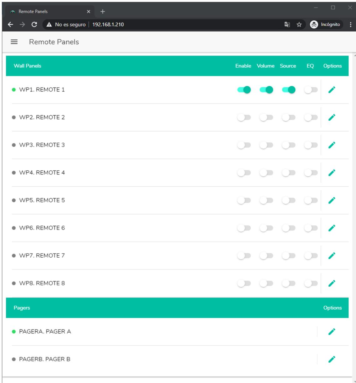
Figure 46: remote control wall panels configuration page
