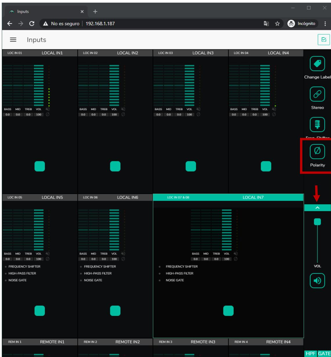
Figure 29: Polarity change of the input signal
