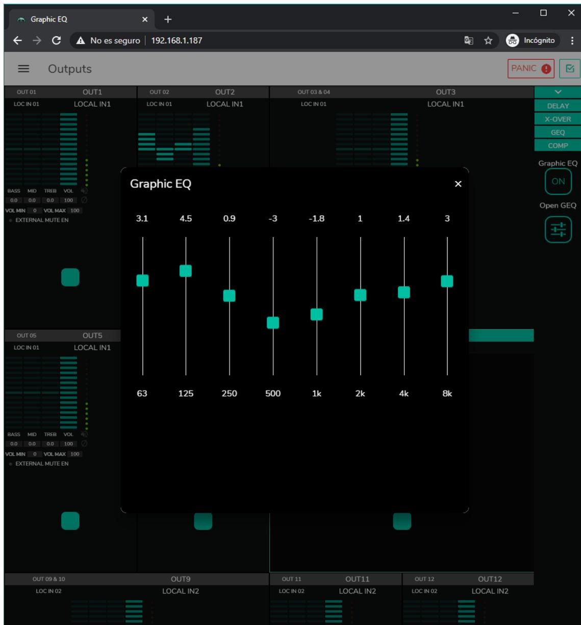
Figure 39: setting the graphic equalizer on an output
